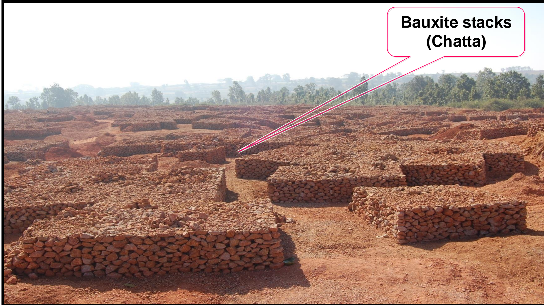
Bauxite Stacking at mine stock yard
